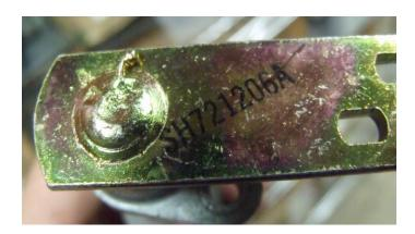
Part number is stamped or painted on the bottom of the pivot in most cases
